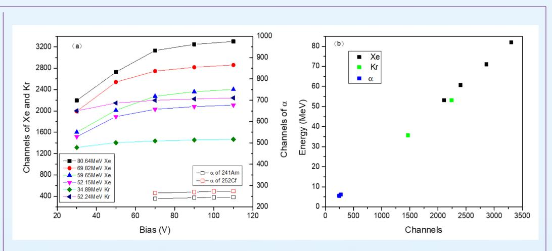
(a) The relationship between bias and channels of Xe  $\sqrt{Kr}$  and  $\alpha$  (b) The Energy response of the SSBD to different particles at operating bias
